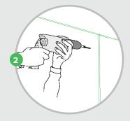
Insert screws with a screwing machine
