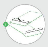
Cut along the two sides with a sharp (Stanley) knife and break along the cutting edge
