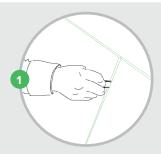
Before finishing joint gaps, make sure the surface of the MAGOXX $^{\scriptsize \circledcirc}$  board is clean and dry
