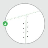
Make sure there is a distance of at least 15–20 mm between the screws and the edges
