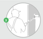
Cover the entire surface with a primer before painting the wall or when in a wet space
