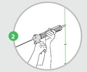
Fill the joints with Bostik ISR 70-03 kit or a similar filling material
