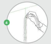
Apply alkali-resistant finishing tape to cover the joint gaps
