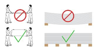
Care should be taken when handling heavy boards. The boards are non load bearing.
