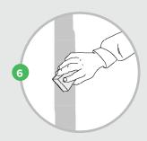
Create a smooth surface by using a sanding block to feather each layer of joint paste. Add additional filler material if necessary
