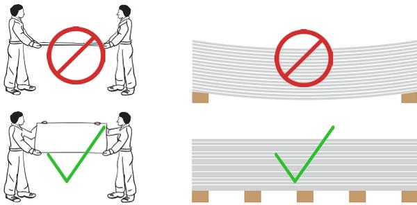
Care should be taken when handling heavy boards. The boards are non load bearing.
